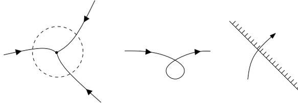
**Fig. 2** The vector fields produced avoid the concentration of agents within any one control volume (dashed circle) (left), paths with local loops (center), and collisions with the boundary of the complex (right).
