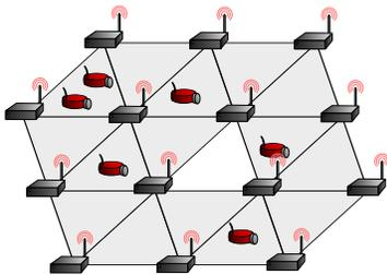
**Fig. 1** Multiple mobile robots (red) execute distributed patrol strategies in a triangulated environment with the help of wireless base stations (dark gray).
