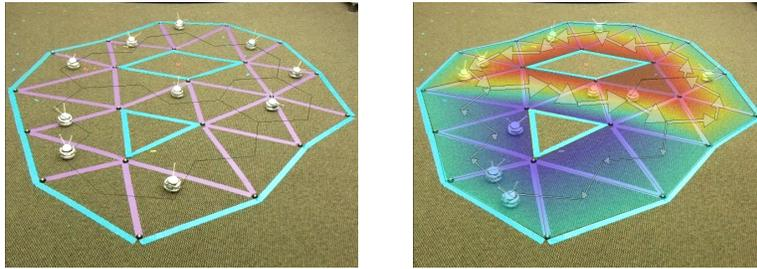
**Fig. 5** Khepera III mobile robots in a simplicial complex (left) (internal edges are shown in purple and boundary edges in blue), and robots moving in the same complex according to a streamfunction, overlaid (right).
